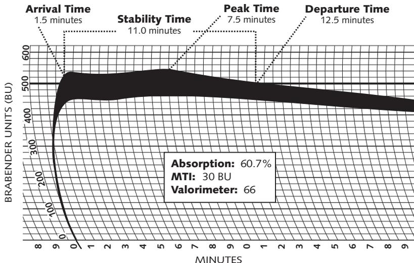
**Arrival Time** The time required for the curve to reach the 500 Brabender Unit (BU) line. Indicates the rate of hydration of the flour.
